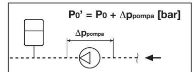
$$Pa' = P_0 + \Delta p_{pompa} \text{ [bar]} + 1 \text{ bar}$$
