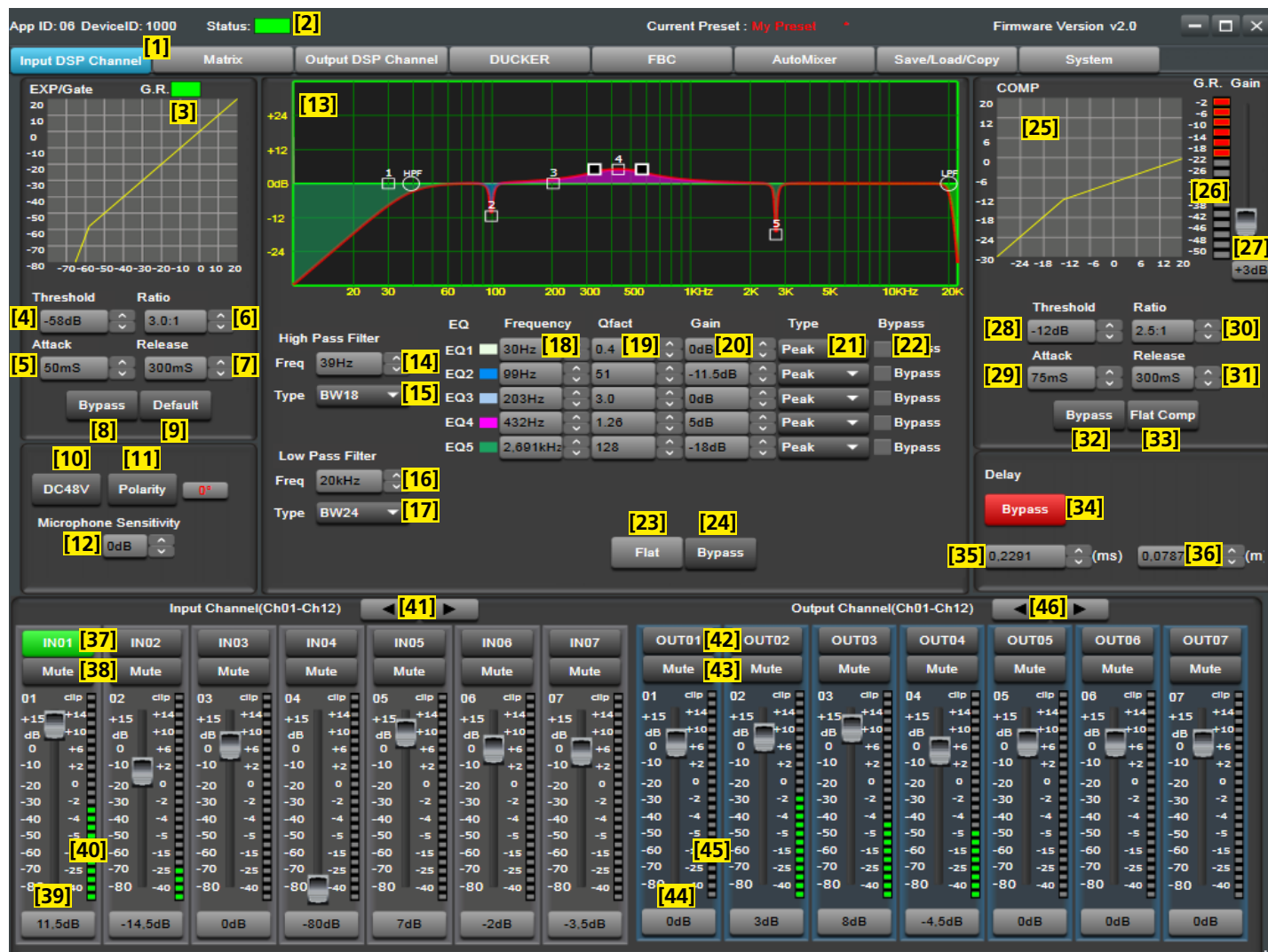
Fig. 20 View "Input DSP Channel"
